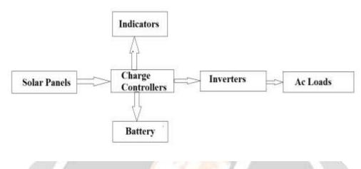
(Block diagram for portable solar power plant)
