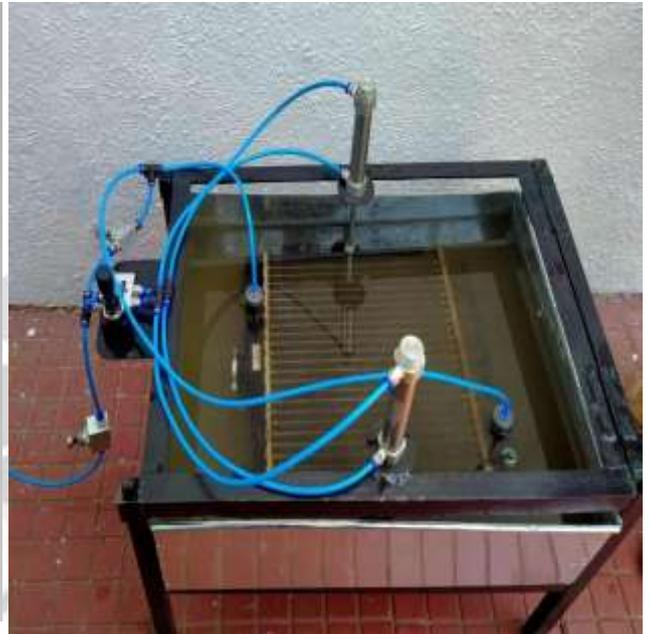
Concept of Radiator and Evaporator leak testing machine.
