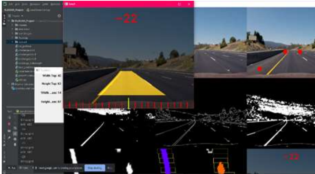
Fig -4: Output visual for a test video showing all the steps in lane detection procedure.
