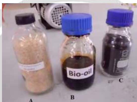
Fig 10: a): Wooden shavings of Dried Red oak fine quality; (b) Bio-oil after the recovery; (c) Bio-char of Pyrolysis of Lignin biomass.
