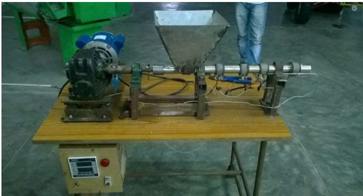
Fig. 1 Plastic extruder after fabrication
