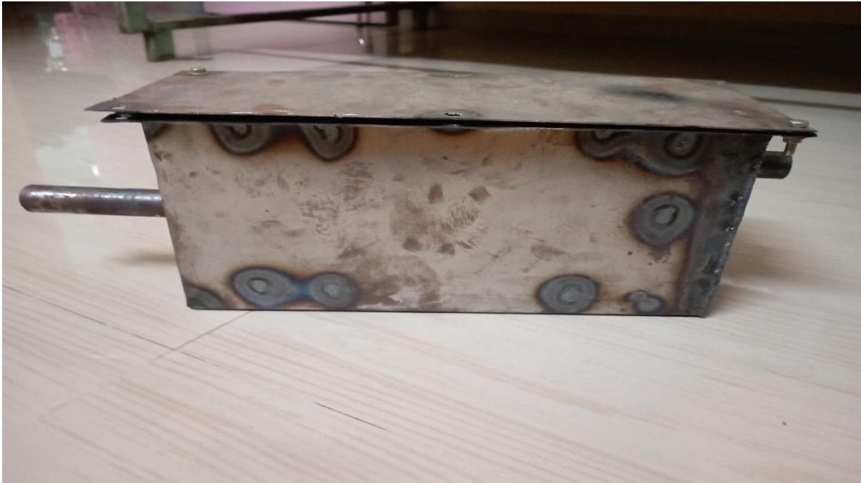
Fig . External View Of Adsorption Unit
