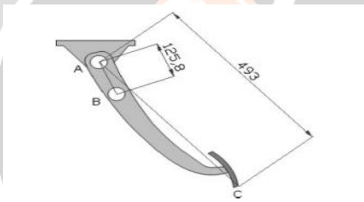
**Fig. 3 Geometric parameters of the brake pedal in millimetres**
