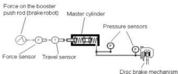
**Fig. 5 The brake system configuration at stage 2**
