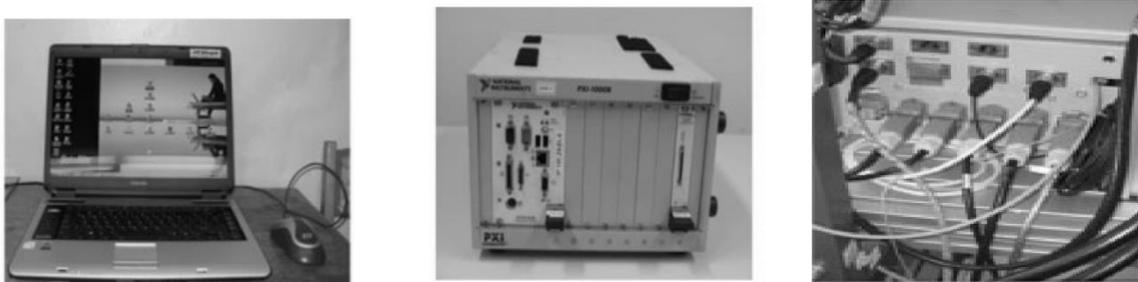
**Fig. 2 Measurement system:** (a) laptop with suitable software; (b) real-time computer; (c) signal converter
