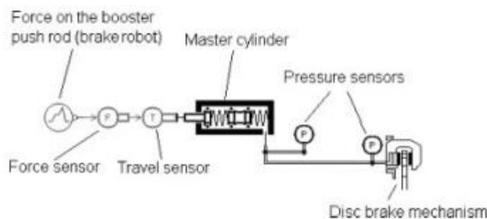
Fig. 6 The brake system configuration at stage 3
