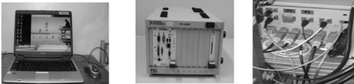
**Fig. 2 Measurement system:** (a) laptop with suitable software; (b) real-time computer; (c) signal converter
