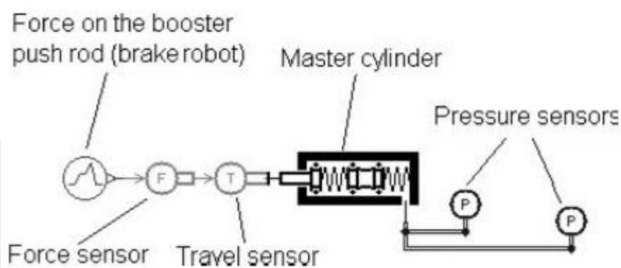
Fig. 7 The brake system configuration at stage 4
