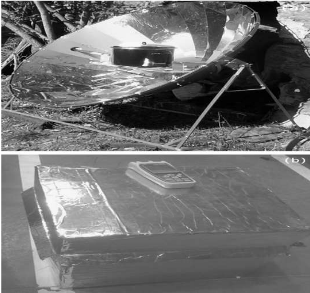
Fig-1 Cooker B in operation showing the focused sun on the utensil. (b) Insulating box closed and instrumentation.
