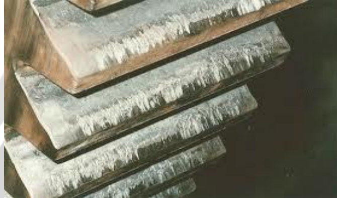
Fig.1. Gear scuffing Effect
