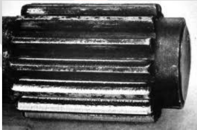
Fig.2. Effect of Gear sticking
