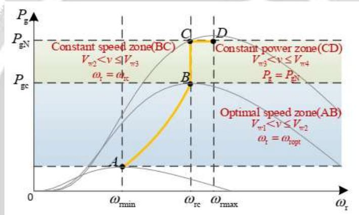
Fig. 4. Power characteristics of DFIG
