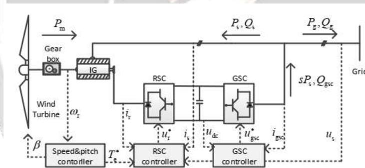
Fig.3. Schematic diagram of DFIG
