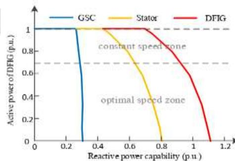
Fig. 5. Reactive power capability of DFIG
