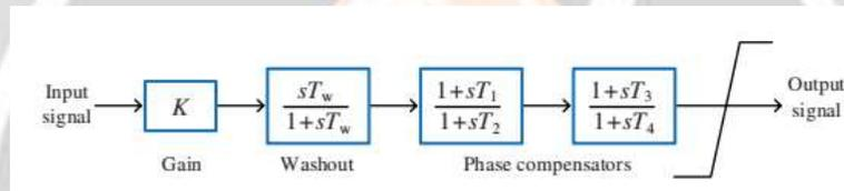
Fig.2. Structure of POD
