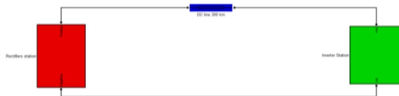
Figure 4.1: MATLAB simulation model for hvdc line power system includes rectifier station subsystem, inverter station subsystem and dc transmission line
