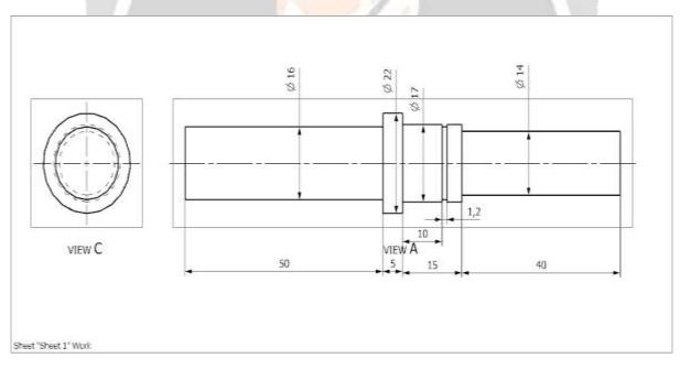
$\begin{array}{ll} Material \ of \ shaft \ EN24 \ allowable \ stress = 144 \ N/mm^2 \\ \Rightarrow \ T \ design \ = 1.28 \ Nm \\ Maximum \ theoretical \ torsional \ shear \ stress \ ( \ f_{\ act \ )} \ = 2.37 \ N/mm^2 \\ As; \ fs_{\ act} < \ fs_{\ all} \ , \ Input \ shaft \ is \ safe \ under \ torsional \ load. \\ \mbox{Analysis of input \ shaft :} \end{array}$
