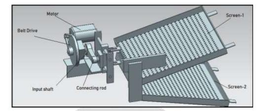
DESIGN INPUT DATA ELECTRIC MOTOR DETAILS POWER= 100 WATT SPEED = Variable( 0-9000 )rpm Design Torque (Tdesign) = 1.28 N.m
