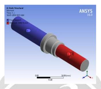
The shaft is fixed at the pulley end and the torque of 1.28 N-m is applied at the end where eccentric is mounted
