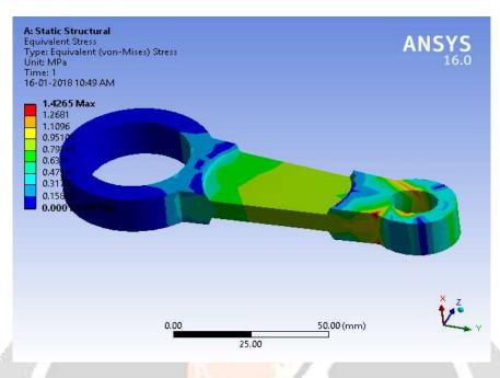
The maximum von-mises stress induced is 1.4265 Mpa which is well below the permissible limit hence the connecting rod is safe
