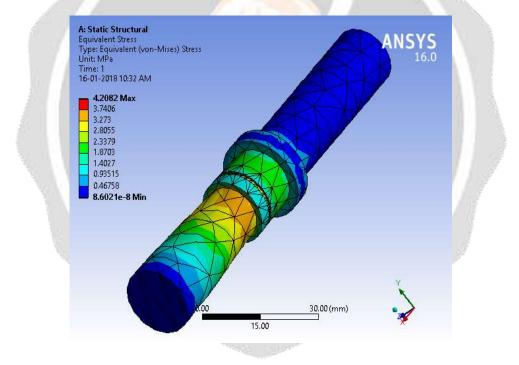
The maximum von-mises stress induced is 4.2 Mpa which is well below the permissible limit hence the input shaft is safe
