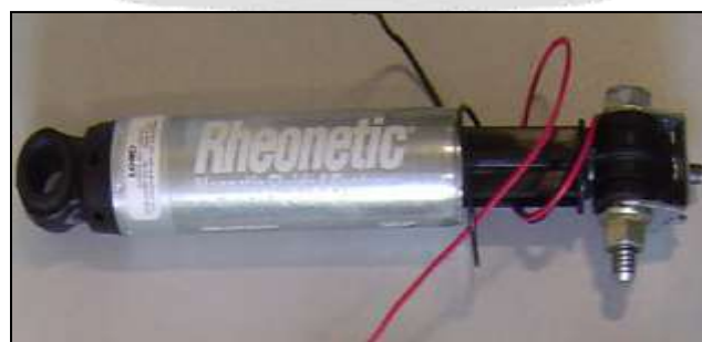
Fig 2: The controllable RD-1097-01 friction damper by Lord.
