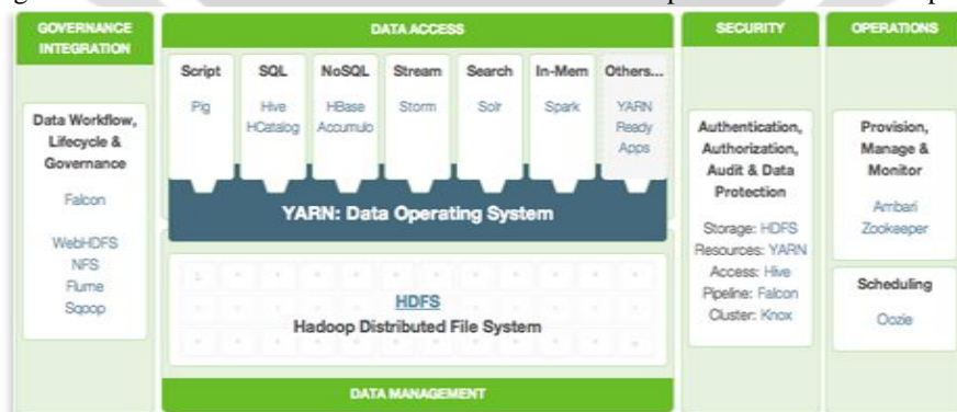
Fig-1: Hadoop architecture [13]
