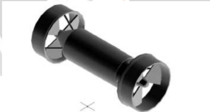
Fig - 2: Double-sided thruster of Minerva
