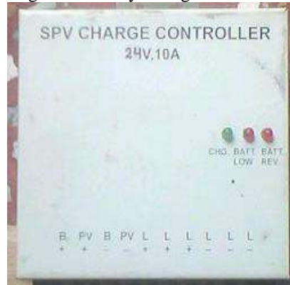
Fig no. 2. Solar Charger Controller
