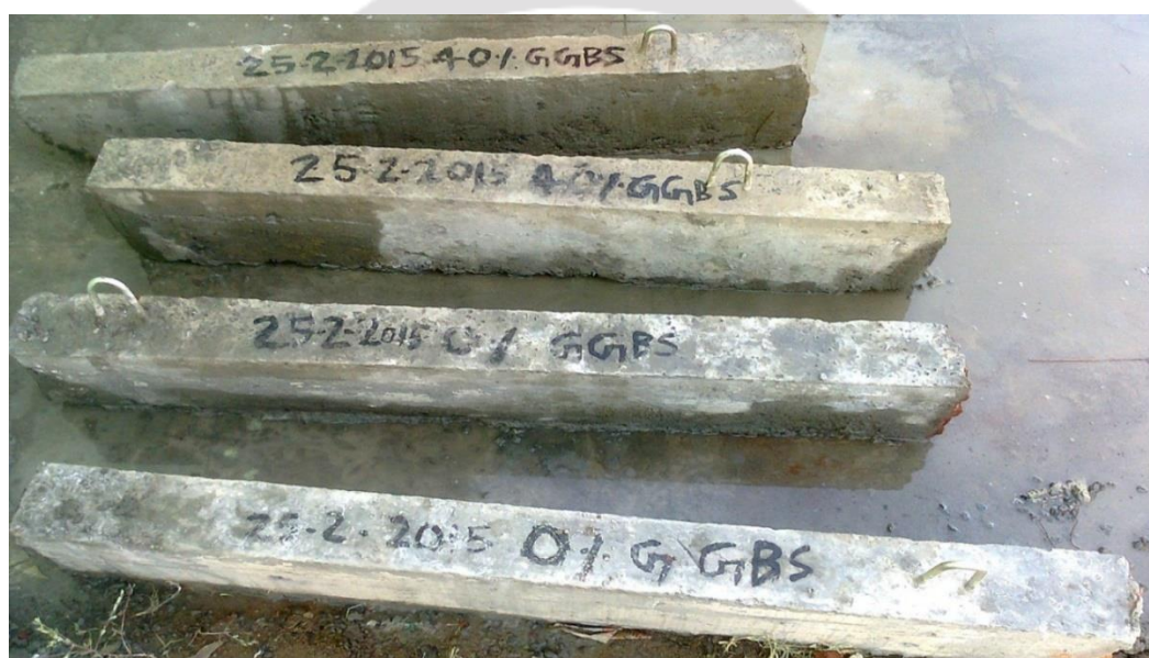
Figure 4.2.5 Casted Beam specimens
