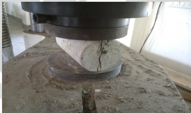
Figure 5.3 Placing and Splitting of Cylinder
