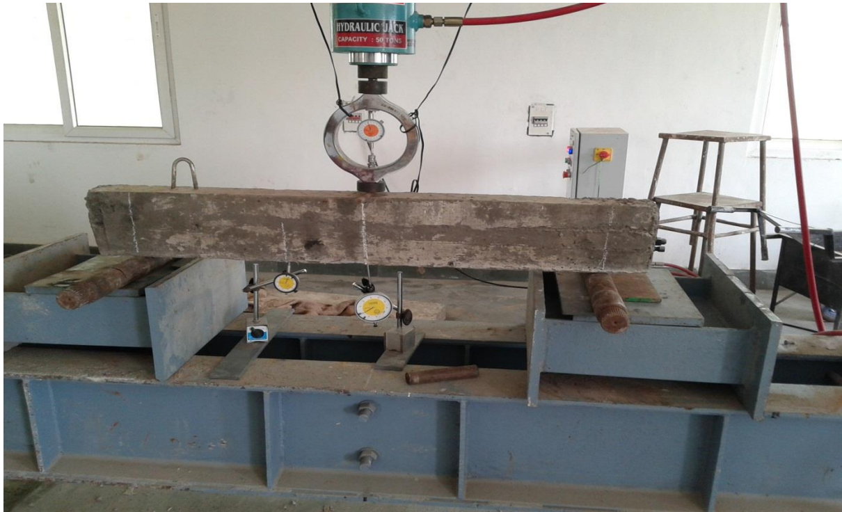
Figure 4.2.6 Test setup for flexural test
