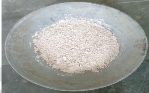
Figure 2.2 Ground granulated blast furnace slag
