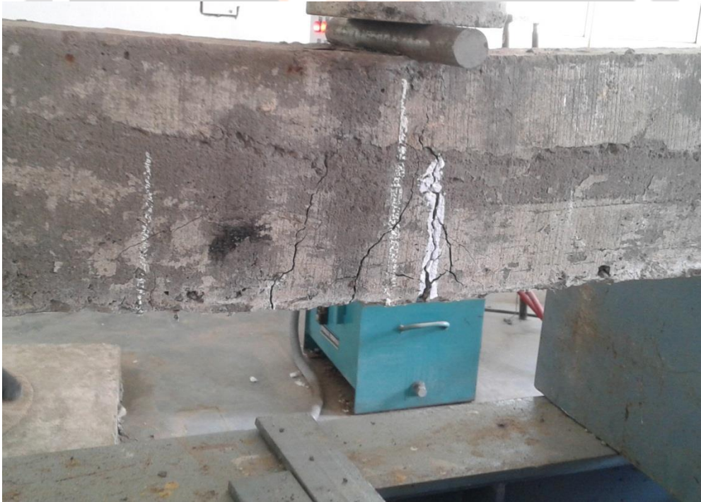
Figure 5.9 Failure of beam specimen S1
