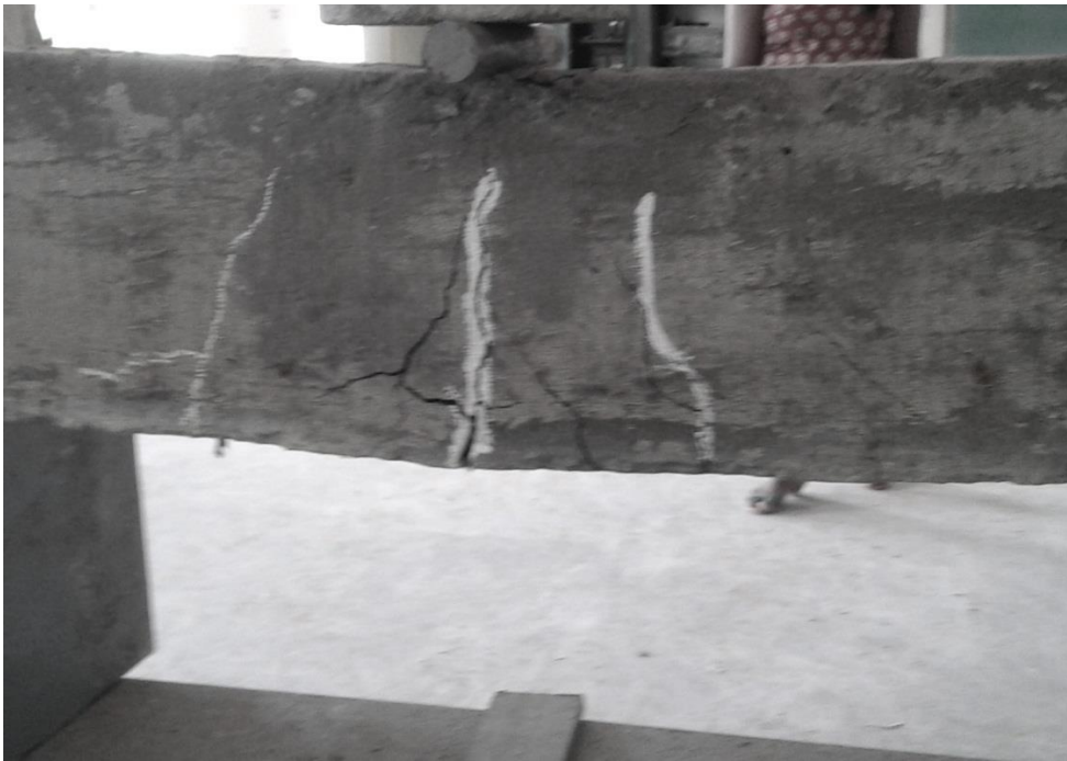
Figure 5.10 Failure of beam specimen S5
