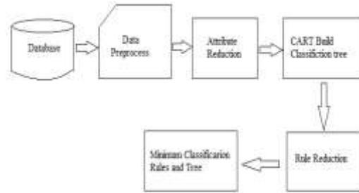
Fig. The basic process of the improved algorithm R2-CART
