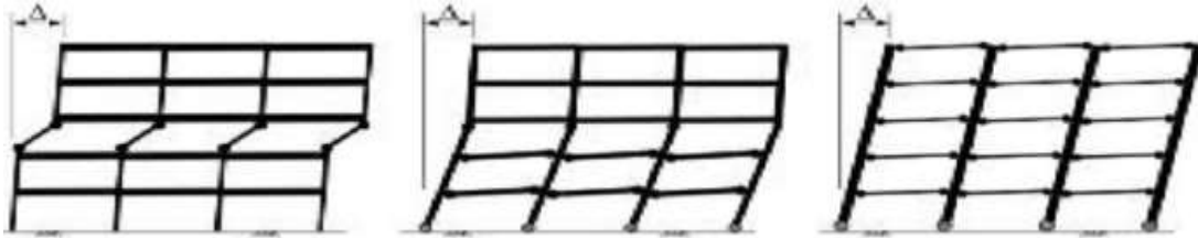
Fig: 4: Story mechanism Intermediate mechanism Beam mechanism (Reference: Moehle et ai., 2008)
