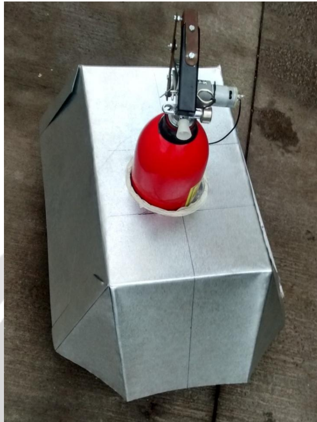
Fig. 7- Working model of Fire extinguishing robot
