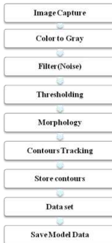
Fig.3 Flow Diagram of our Detection Steps
