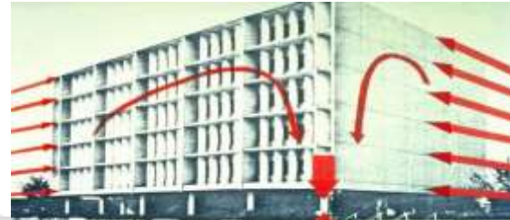
Fig.4 Development of inertia forces
