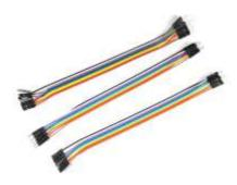
male to male wire are used to connect the connection in breadboard to ardiuno and buzzer.and male to female wire is used to connect the ultrasonic sensor.ardiuno,breadboard etc.
