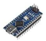
The Arduino Nano is a small Arduino board based on ATmega328P or ATmega628 Microcontroller.
