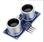
and ultrasonic sensor is used to sence the object at the distance
