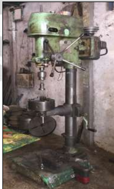
Fig -2: Drilling machine
