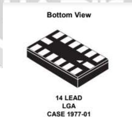
Fig -4: Bottom view of MEMS sensor
