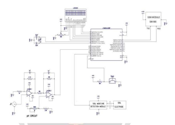
Circuit Diagram- Smart sensor based soil monitoring system
