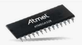
oscillator, and five software selectable power saving modes. The device operates between 1.8-5.5 volts. The device achieves throughput approaching 1 MIPS per MHz.
