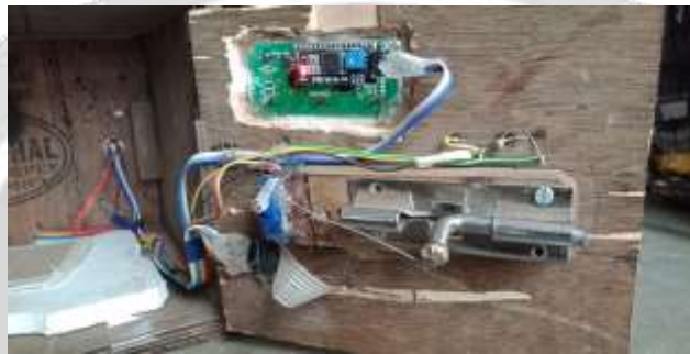
Fig.3 Servo Motor And Latch Arrangement(with I2C Module)
