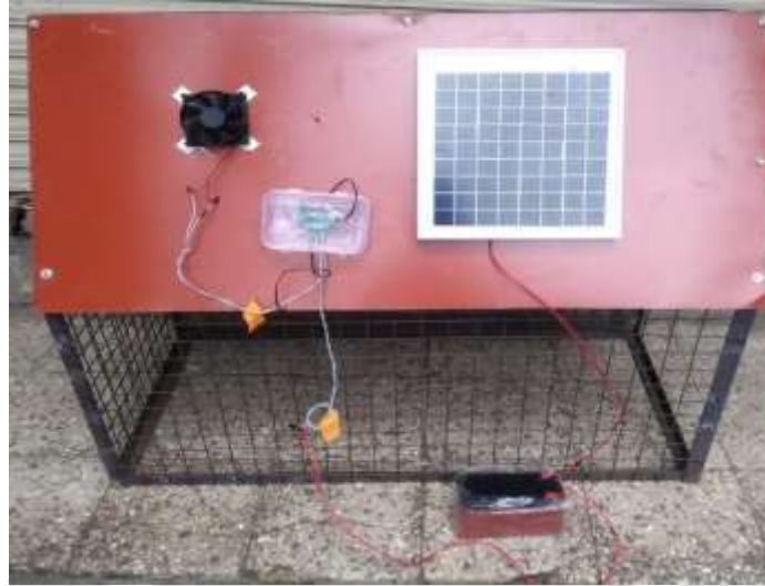
Fig. 3.9: Solar Operated Cooling System for Poultry Shed (Actual Model)
