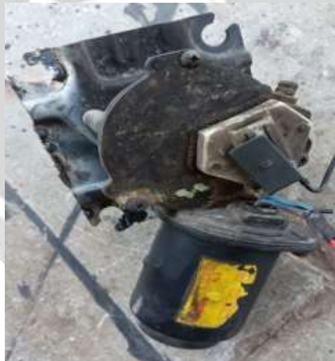
Figure 2: 12V DC motor detached from car wiper.
