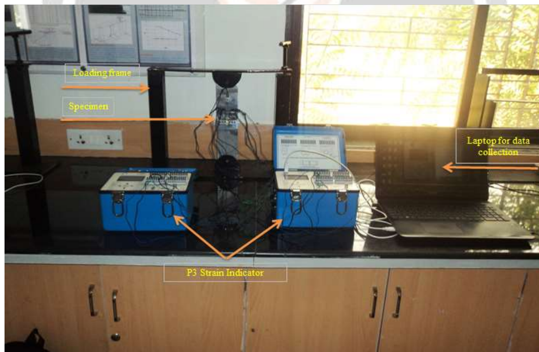
Experimental setup for elliptical cutout (Electrical strain gauge method)
