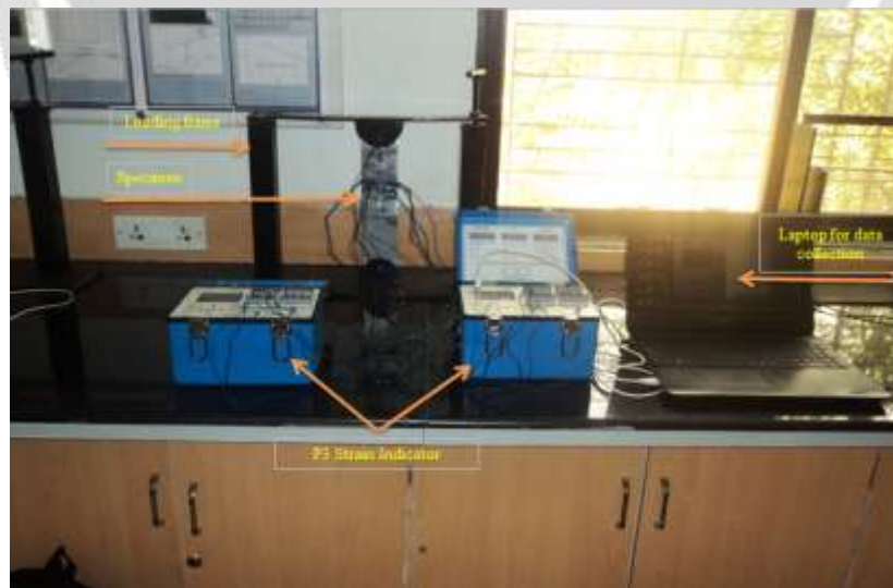
Fig-5 Experimental setup for square cutout (Electrical strain gauge method)
