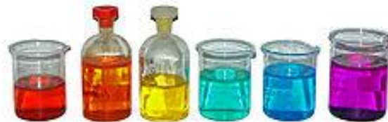
From left to right, aqueous solutions of: \text{Co}(\text{NO}_3)_2 (red); \text{K}_2\text{Cr}_2\text{O}_7 (orange); \text{K}_2\text{CrO}_4 (yellow); \text{NiCl}_2 (turquoise); \text{CuSO}_4 (blue); \text{KMnO}_4 (purple).
