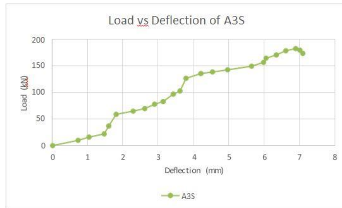
Fig 6.3 Experimental Result of Load Vs Deflection Curve for RC Beam with Three Layer of Aluminium Alloy
