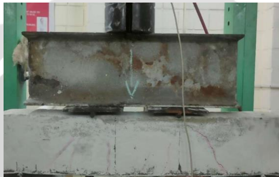
Fig 5.11 Beam with Two Layer of Aluminium Alloy Plates at Bottom
