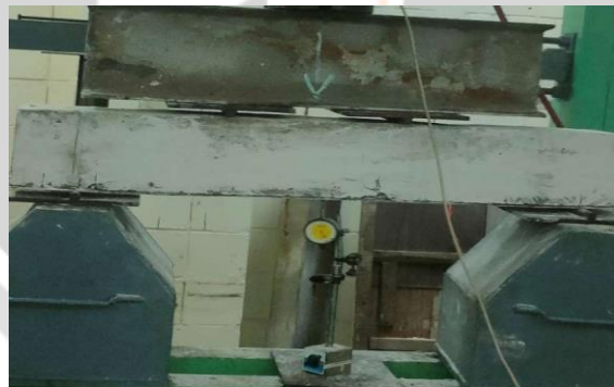
Fig 5.12 Beam with Three Layer of Aluminium Alloy Plates at Bottom
