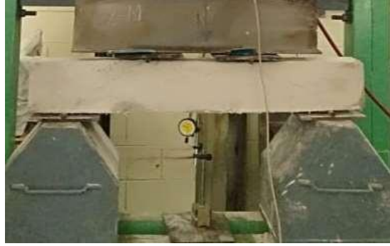
Fig 5.10 RC Conventional Beam
