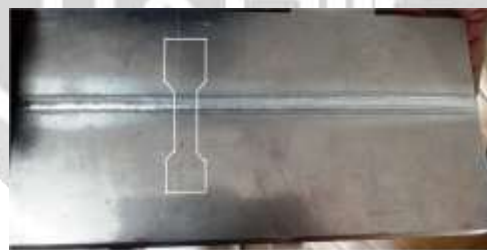
Fig - Tensile test specimen Preparation
