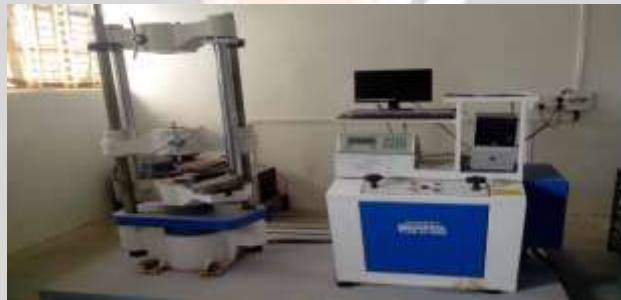
Fig -Process setup for tensile test
