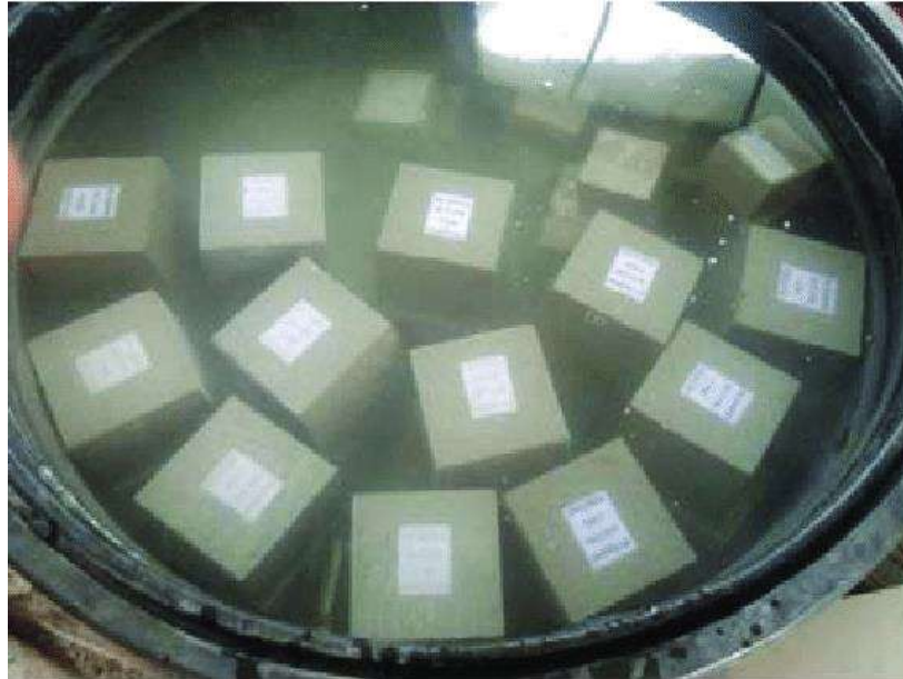
Fig-2: During Chemical curing of beams
