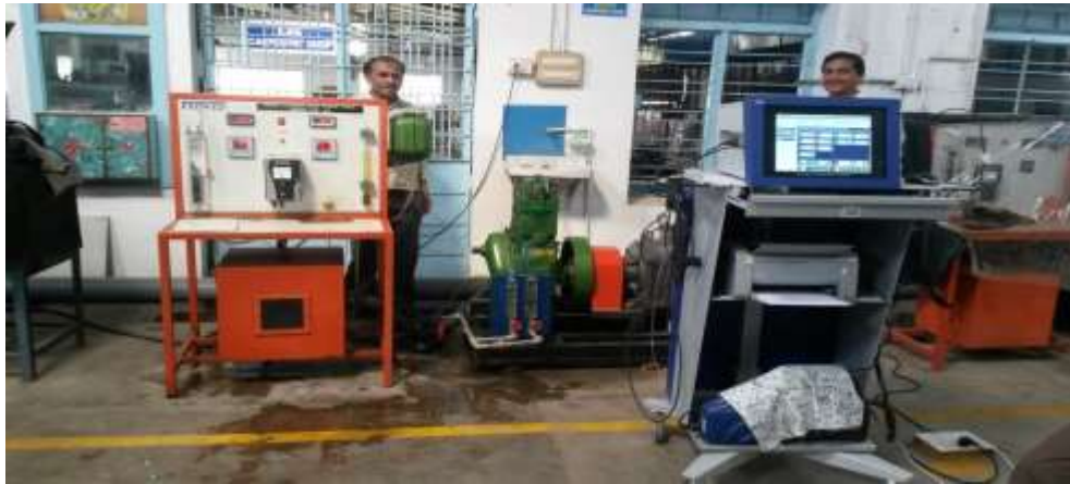
Figure: 2.6 Diesel Engine Test Rig with AVL DiTEST (Exhaust gas analyzer)
