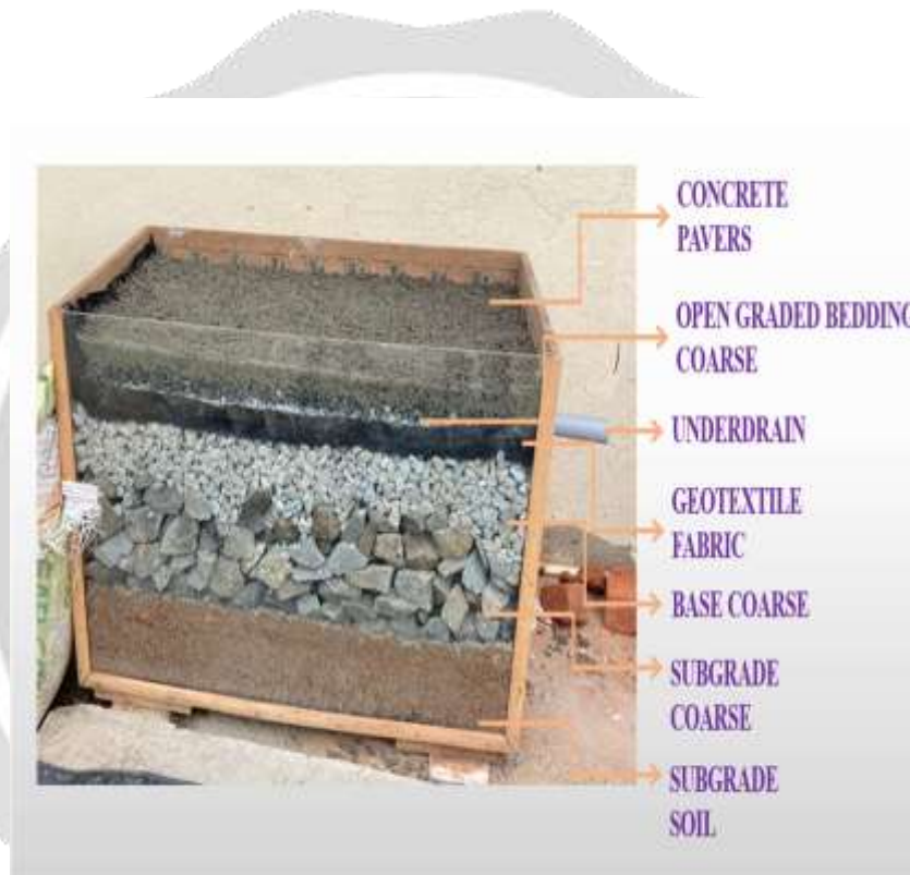
Fig -2.5: Model of C/s View of pavement
