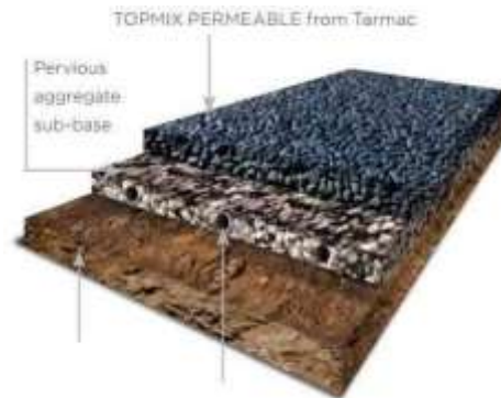
Fig -1.1: Tarmac Concrete layer
