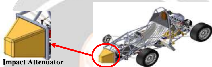
Fig. 1 Impact attenuator attachment to front bulkhead.
