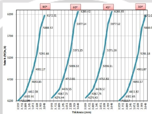
Chart 3 Tube Side Heat Transfer Coefficient vs Tube Thickness
