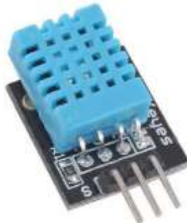
Fig :Humidity sensor
