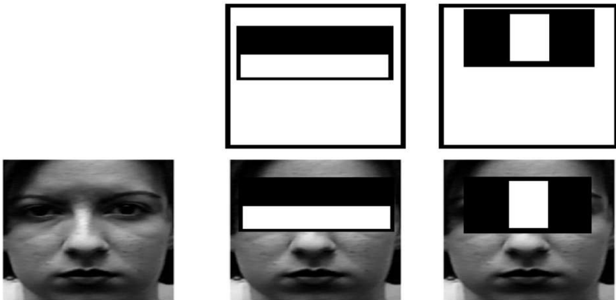
Features selected by the AdaBoost learning algorithm in a face from the CK+ database.
