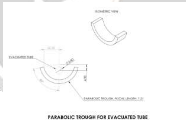
Fig. 3 Specifications of parabolic trough
