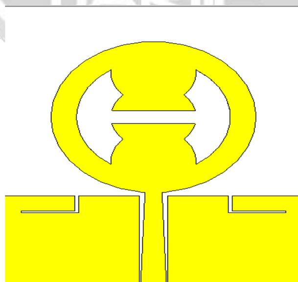
FIG: DESIGNED ANTENNA SIMULATED IN CST SOFTWARE
