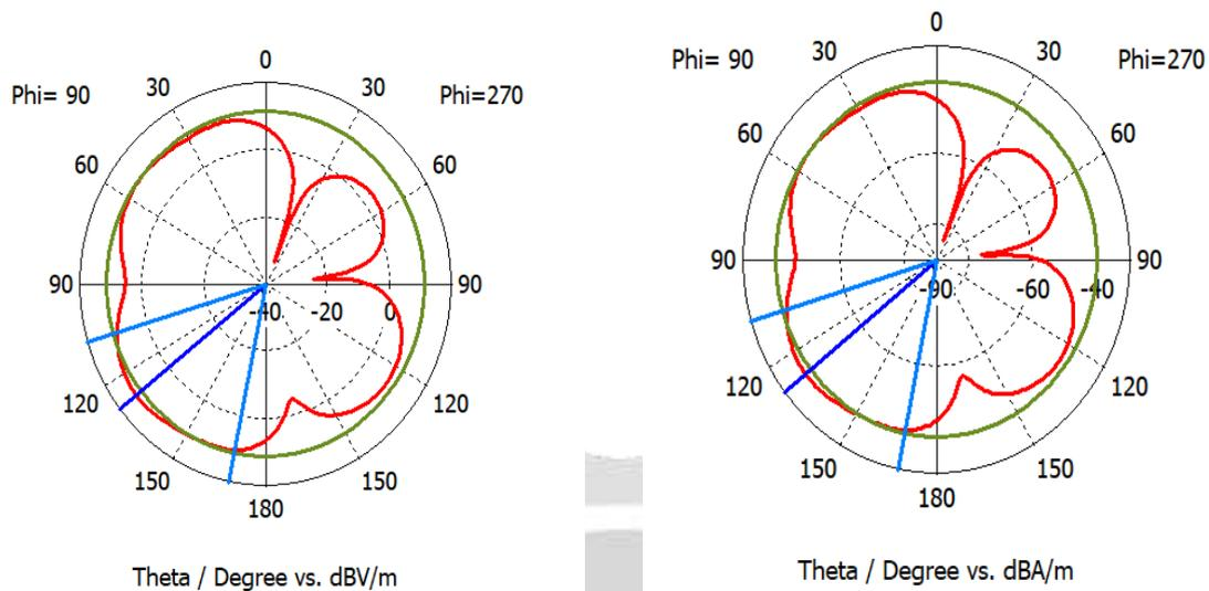
FIG: E-Field and H-field patterns at  $f=10\text{GHz}$
