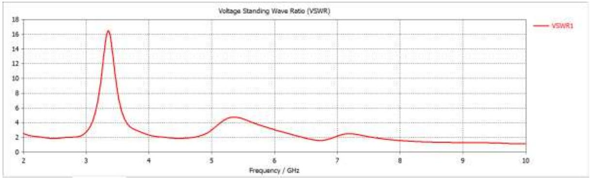
FIG: VSWR obtained for the Designed Antenna with Notch Bands at 3.5GHz and 5.5 GHz
