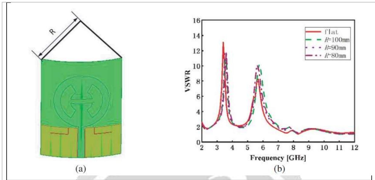
Figure 1. Performance of the bent antenna. (a) Diagram of the bending test. (b). Simulated VSWRs with different R.
