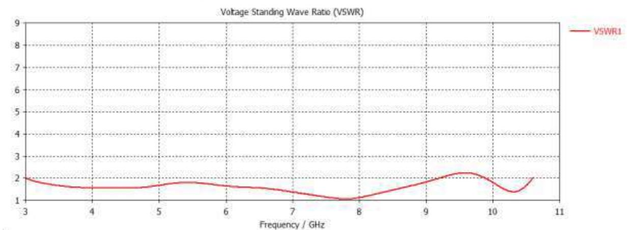
Figure 2. VSWR of Ultra Wide Band (UWB) Antenna
