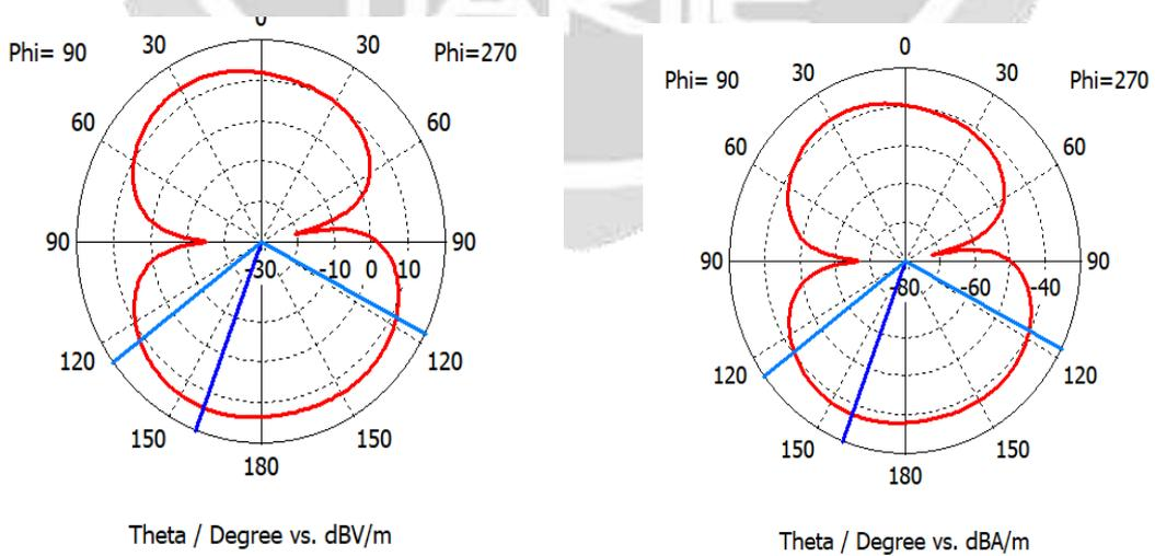
FIG: E-field and H-field patterns at 5.5GHz
