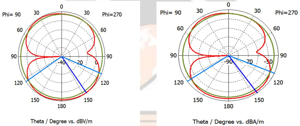
FIG: E-field and H-field patterns at 3.5GHz
