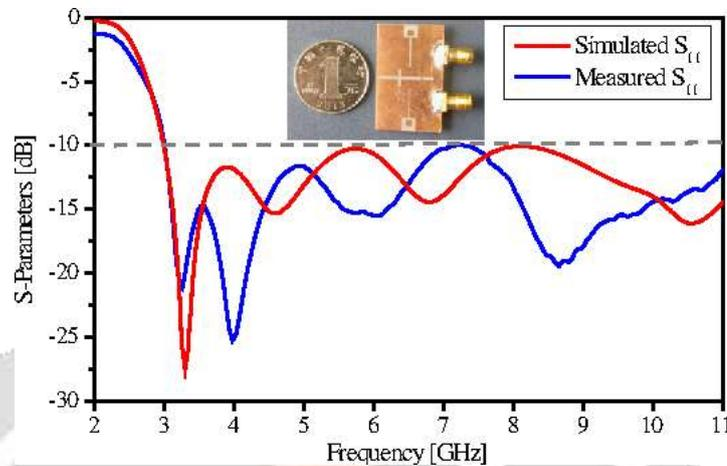
Figure 3. S-Parameters plot of Ultra wide band Antenna
