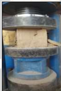
Fig -2 : Compression testing of adobe specimen
