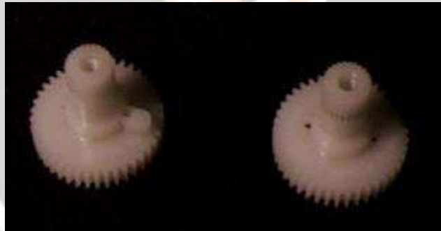
Fig -5: An unmodified (left) and modified output shaft gear
