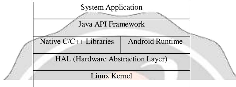
**Fig 1.3 Android Platform Architecture**<sup>[6]</sup>
