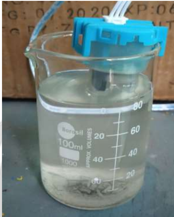
Fig :4.4 River water sample Turbidity checking in beaker
