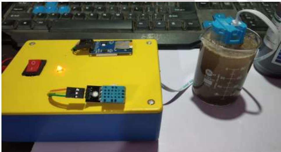
Fig :4.18 Data Logger Used In this Experiment For Finding total suspended solids (TSS) in NTU unit.
