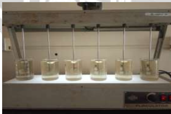
Fig-12: Jar test using Peanut seed powder
