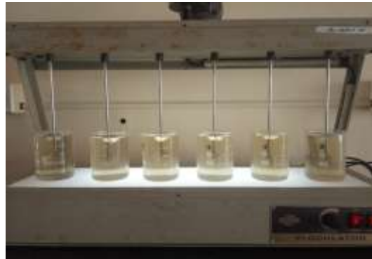
Fig 10: Jar test using chickpeas as coagulant
