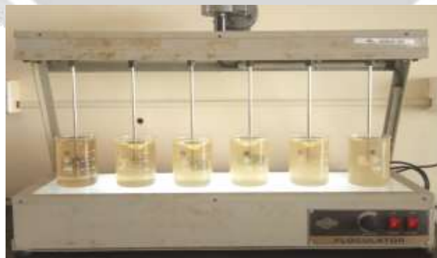
Fig-9: Jar test using Aloe Vera
