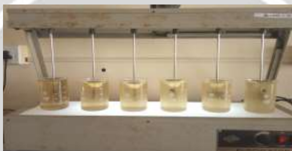
Fig-11: Jar test using Palmyra palm
