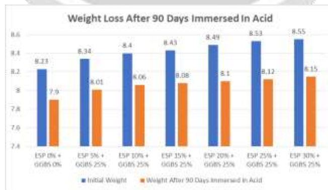
Fig. 10 Weight Loss After 90 Days Immersed In Sulphate Acid
